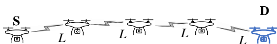
Fig. 3. An example of data transmission route from S to D, including links L1, L2, L3 and L4.
