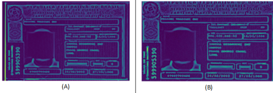
Fig. 2. The boarder artifacts visible in screen recaptured images generated by the Meijering filter. Images are shown in the viridis colour space, which is the default for matplotlib. (A) Original. (B) After cropping.
