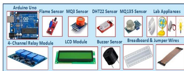
Fig. 8. The hardware components for the proposed chemical lab safety stage.
