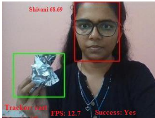
Figure 5. Person detection along with object using CSRT tracker.
