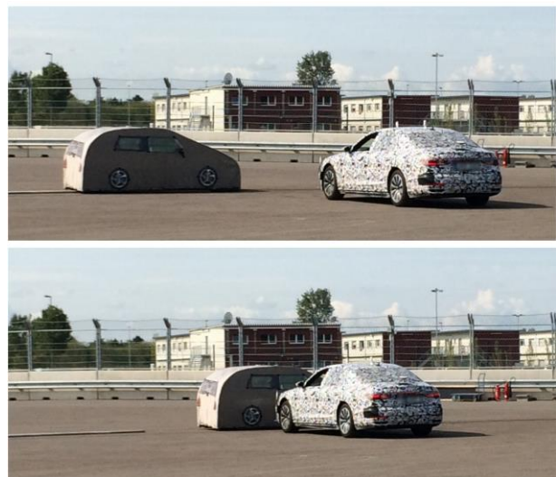
Figure 1. Crash test with dummy vehicle on the CARISMA outdoor facility at Technische Hochschule Ingolstadt
