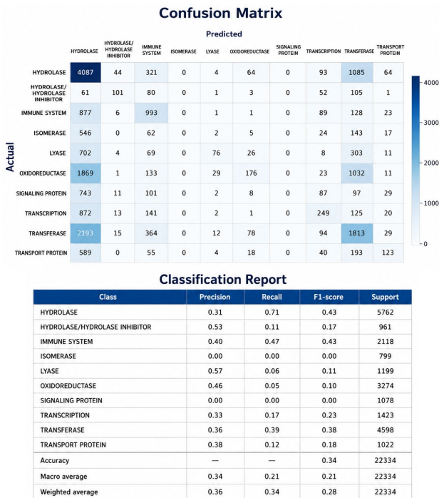
Fig. 7. Confusion matrices and classification report for PSSM encoding based on a CNN classifier.
