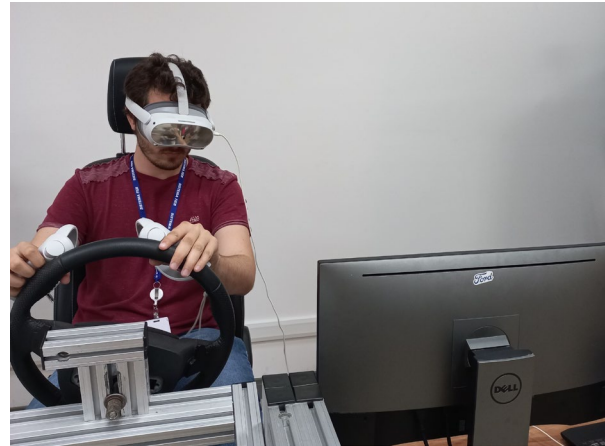
Fig. 11. Aligning the physical and the virtual steering wheel.
