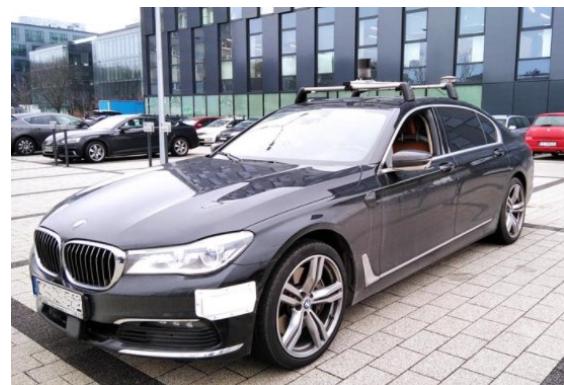
Fig. 1. Typical data recording vehicle used during Advanced Driver Assistance Systems (ADAS) system development.
