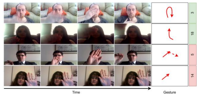
Fig. 5. Misclassified sequences for gestures 3 (pulling hand in), 18 (swiping up), 5 (pushing hand away), and 14 (stop sign). The trajectory of the gestures is also shown to better understand the differences between them. Problematic gestures with the same label color underscore potential confusion.
