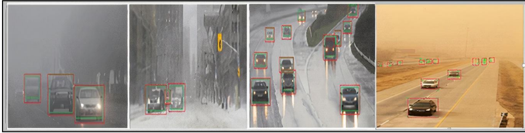
Fig. 4. Accurate identification of on-road vehicles utilizing the proposed approach on test images sourced from the DAWN dataset under fog, snow, rain and sandstorm conditions.
