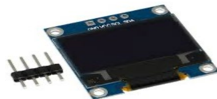
Fig. 6. OLED display (SSD1306) for real-time physiological data visualization and encryption output.
