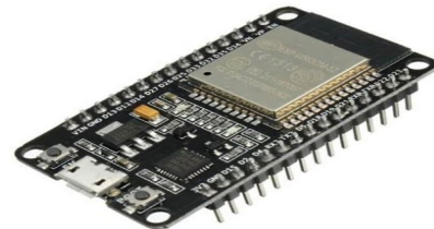
Fig. 5. Microcontroller ESP32-WROOM-32 with built-in WIFI and Bluetooth for edge cryptographic processing.
