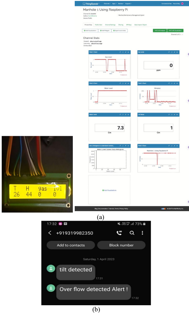
Fig. 3. Output results. (a) output result graphs from Manhole 1 Raspberry Pi (b) tiltsensor output and alert mechanism through SMS.
