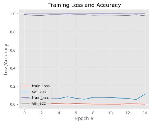
Figure 10. EfficientNet-B0 accuracy/loss curves for the train and test datasets of D0 during the unfrozen process.
