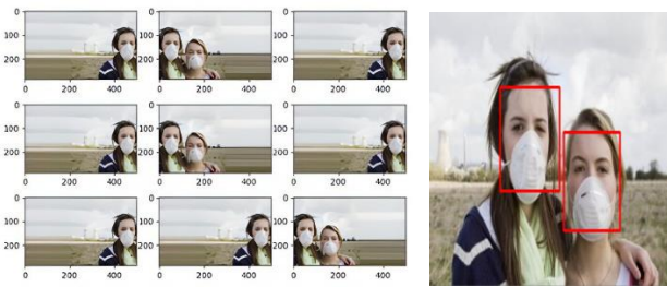
Figure 2. Data preprocessing phase: (a) Data augmentation, (b) (Region of interest) ROI detection.
