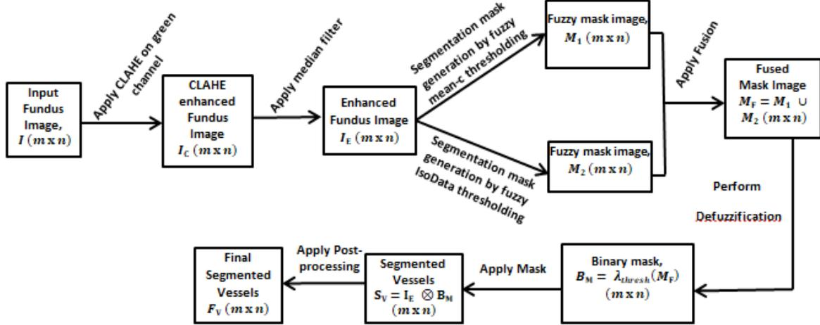
Figure 1. Block diagram of the proposed approach.
