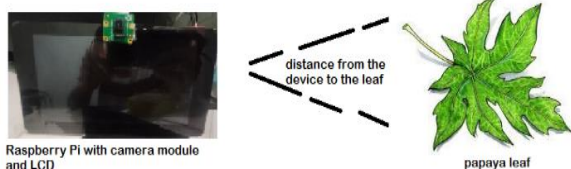
Figure 2. Image capturing setup.
