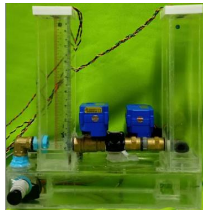
Figure 8. Level control process prototype.
