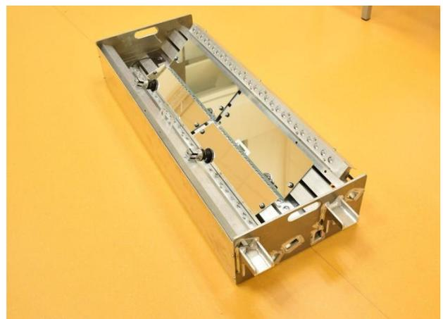
Figure 8. Device used to capture the images. Mirrors are used to increase effective distance from the target.
