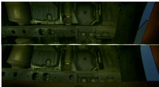
Figure 9. Stereo image of undercarriage captured by one camera and two mirrors.
