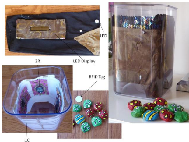
Figure 15. Zigbee-enabled game of Jacks combined with a wearable ZigBee-enabled shirt where children need to answer a question that appears on their shirt by throwing the right 'stone' into the jar
