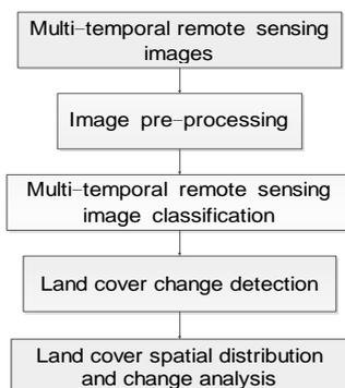
Figure 1. The flowchart of the proposed monitoring method.
