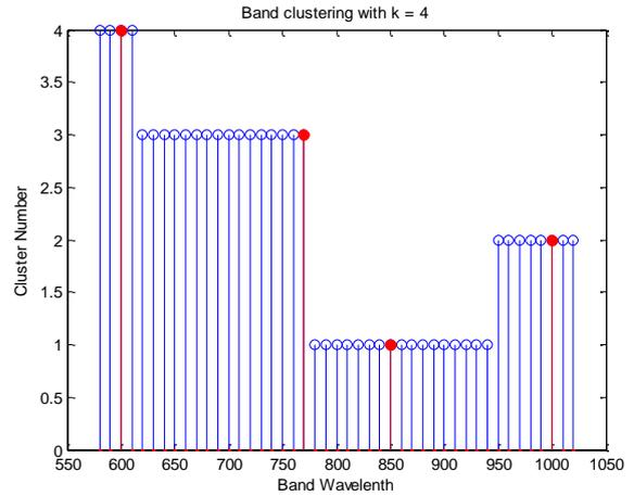
Figure 5. Clustering based band selection with k=4
