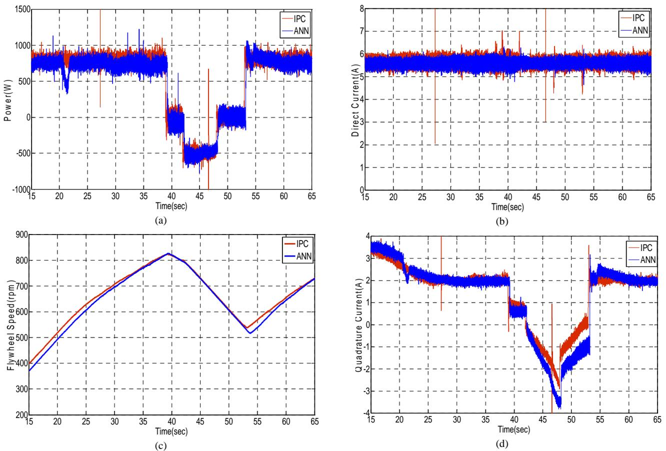
Fig. 7. Experimental results: IPC vs. ANN (a) stator actual power, (b) stator direct current, (c) flywheel speed, (c) stator quadrature current.
